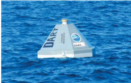
Figure 10-9 Deep-Ocean Assessment and Reporting of Tsunamis System (DART)
